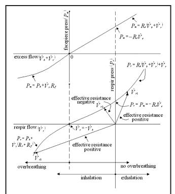
**FIGURE 2.** Pressure-flow diagrams for the PAPR facepiece (above) and the wearer (below); resistance detected by the wearer varies in magnitude and sign.
