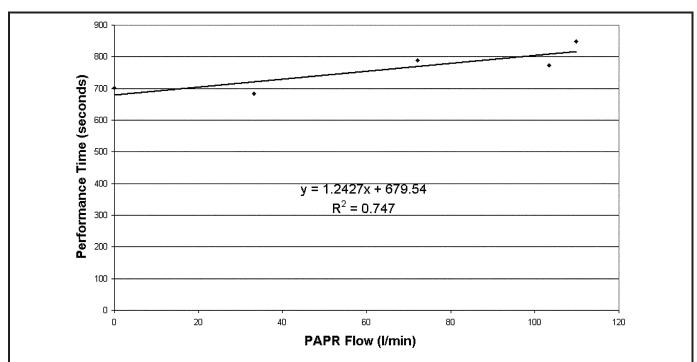
**FIGURE 4.** Average performance times for work at different flow rates. Performance times decreased as flow rate decreased, indicating that inhalation resistance was the most important determinant of performance.
