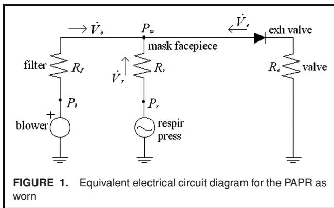
**FIGURE 1.** Equivalent electrical circuit diagram for the PAPR as worn
