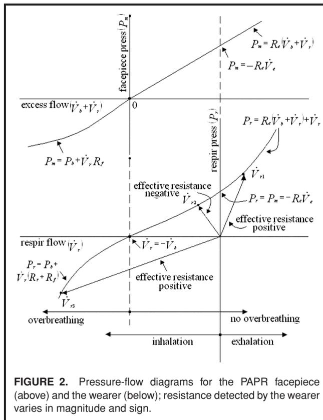
**FIGURE 2.** Pressure-flow diagrams for the PAPR facepiece (above) and the wearer (below); resistance detected by the wearer varies in magnitude and sign.
